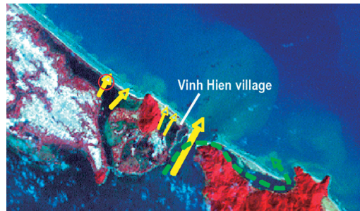
Fig. 3. Thuan An inlet in November 2000 (Green broken line is original waterway before the flood and yellow line shows the flash flow at the flood.)
